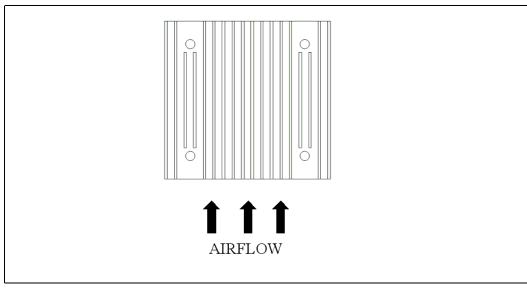
Figure 12. Heatsink Orientation Relative to Airflow Direction
